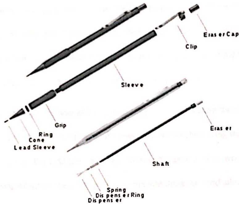
Figure 2: Mechanical Pencil Diagram
